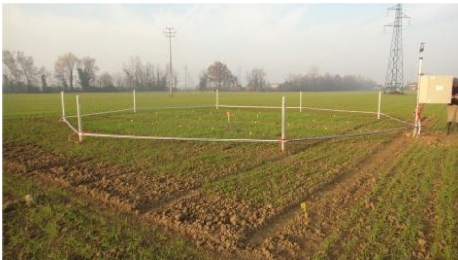
Fig. 3 A picture of the experimental FACE setup in Italy. The FACE unit was used to test and evaluate the performance of the CNR-FACE design and the verification of the new hardware that was developed and then used, including the novel PID algorithm implemented.
