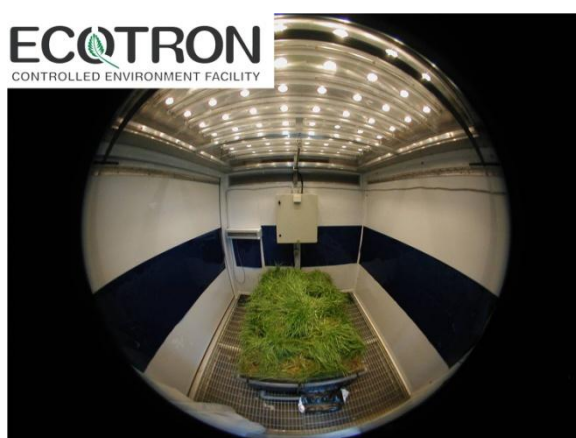
Figure 4.1 The Ecotron – a controlled environment facility designed for community and ecosystem research.
